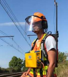
**Fig. above** The system CLARIS connects protection staff and vegetation workers to another via radiotelephony.
