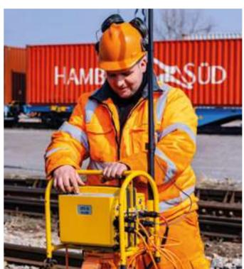
Fig. above The activation point for automatic train detection is composed of the wheel sensor F500-SEN, the connection box F500-AB and the radio transmitter ZFS.
