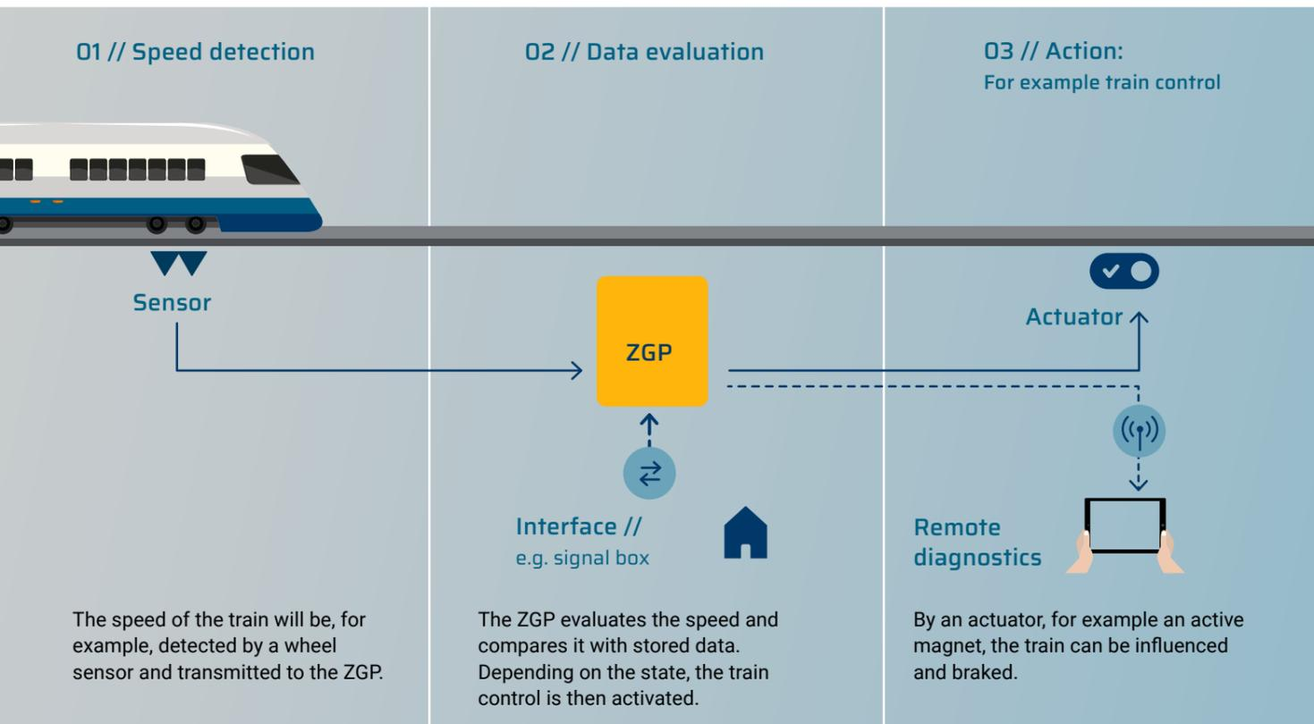
The graphic shows the structure of the system as a velocity testing device with sensor, evaluation and actuator. Other interfaces are possible, for example to the interlocking and for remote diagnostics.
