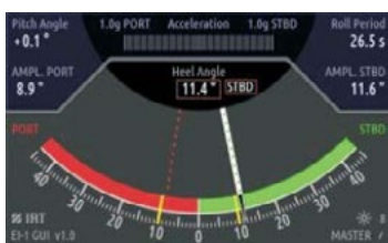
Monitor display with current heel angle (graphic and numeric), current pitch angle, max port and starboard heel as well as horizontal acceleration
