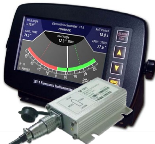
Monitor display with current heel angle (graphic and numeric), current pitch angle, max port and starboard heel as well as horizontal acceleration
